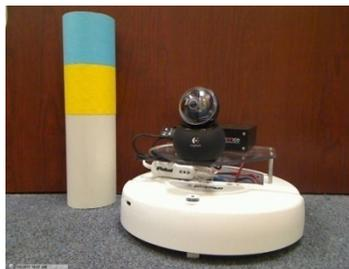
Figure 4: Robot node implemented with an iRobot Create.
