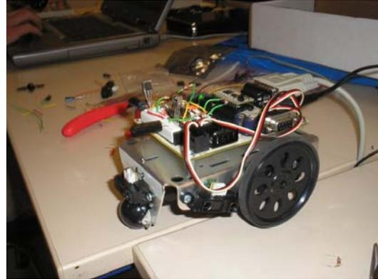
Figure 5: Second prototype robot with IR sensors
