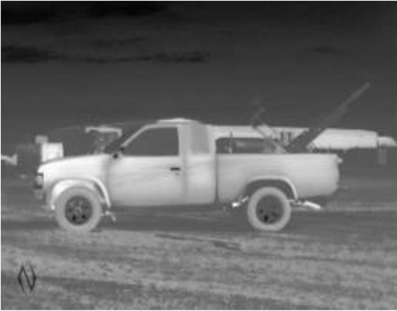
Figure 2. Example FLIR image of a vehicle for use in evaluating a convoy member's ability to recognize other convoy members.
