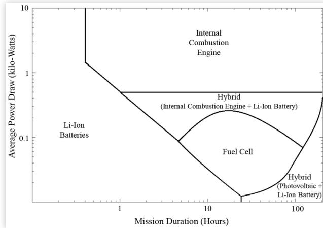
system weight included the weight of the power source, accessories (e.g. alternator), and any necessary fuel. These values were compared between the different technologies to determine the lightest weight option. This analysis focused on a power range from 10 W to 10 kW and a duration from 10 minutes to 200 hours. The results are plotted in [Figure 1](#).
