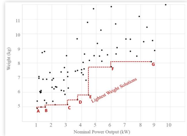
**TABLE 3** Optimal engines identified by the Pareto Frontier analysis displayed in Figure 4.
