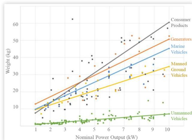
**TABLE 2** Linear approximations for the engine dry weight as a function of power output for different markets
