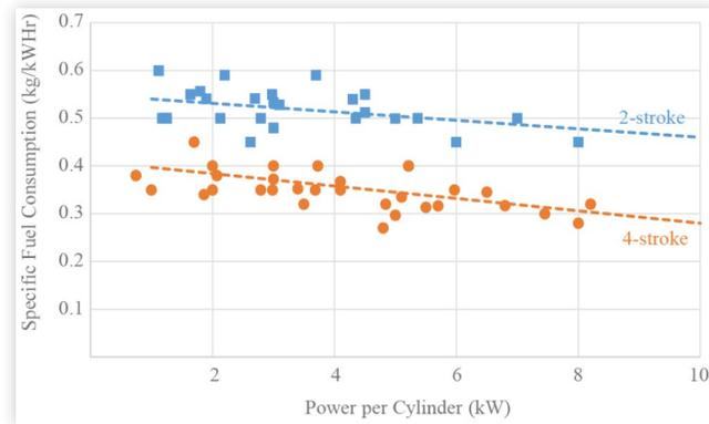
to volume ratio increases. Friction and heat transfer scale with surface area, while power output scales with volume. Therefore, as the cylinder gets smaller, the efficiency decreases and the SFC increases. The size of the engine cylinder(s) scales with the power output divided by the number of cylinders.
