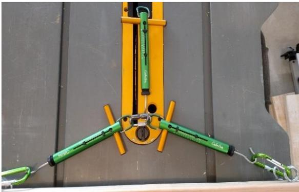
**Figure 5. 30 Degree Connection Angle**
