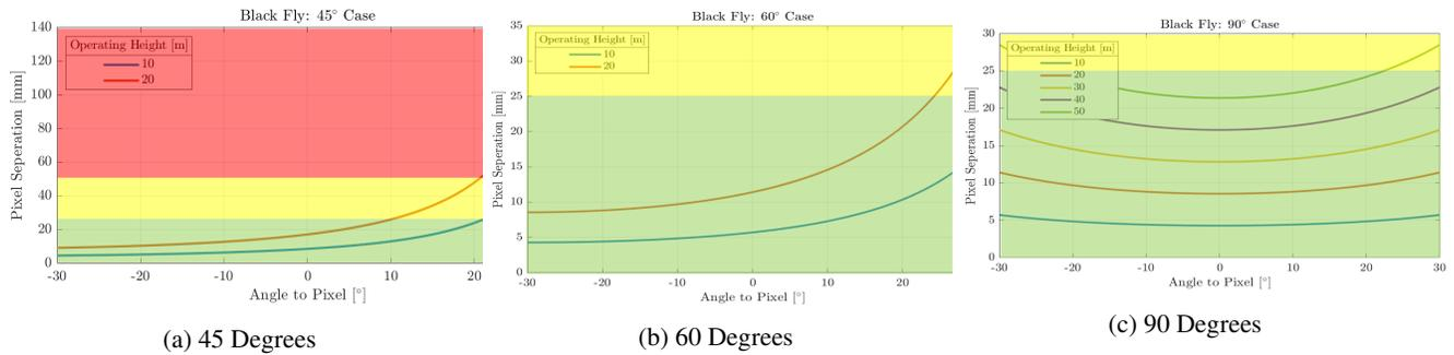
Figure 4. Pixel density requirement for detection at different angles
