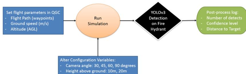
Figure 5. Flowchart of Testing Methodology
